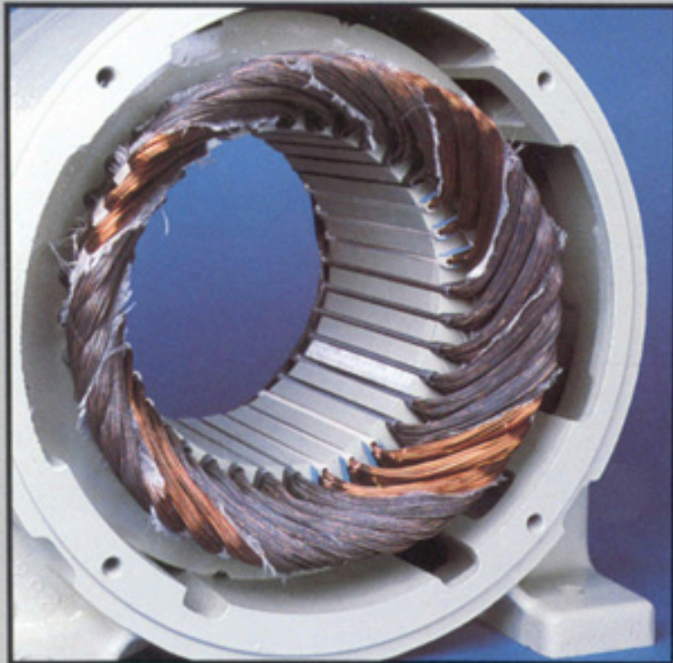
1 Winding Single-Phased (Y - Connected)
