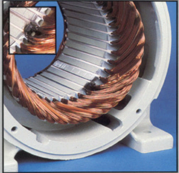
6 Winding Grounded at Edge of Slot
