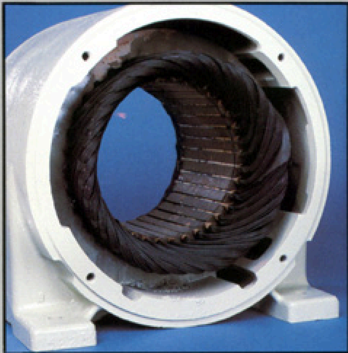
10 Winding Damaged Due to Overload
